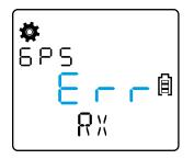
If the transmission test is not successful, the message "**Err**" will be displayed. The main causes can be: absence of the antenna, antenna not powered, antenna too far away. If the antenna is present, install an appropriate number of Type 1Y.E8 range extenders between the antenna and the time switch.
