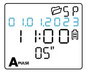
図日 1 日 3 5 1 月:日日 05" Press and hold up to set start date (**ST** - start). Press right or left to move between day, month and year. Press center to continue.
