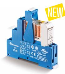
The 48.32.9.024.5060SPA relay interface module is made up of a 50.12.9.024.5000, 2 pole 8 A relay with forcibly guided contacts, mounted on a 95.05SPA socket with a Type 99.02 LED + varistor plug-in module
